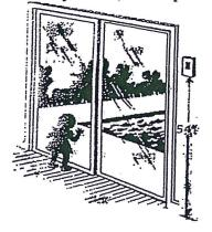
In such cases, the wall of the house is an important part of the pool barrier, and passage through any doors in the house wall must be controlled by one of the following security measures.
