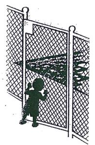
These are the gates people must walk through. Swimming pool barriers should be equipped with a gate or gates, which restrict access to the pool. A locking device must be included in the gate design. Pedestrian gates must open outward and away from the pool and shall be self-closing and self-latching.
